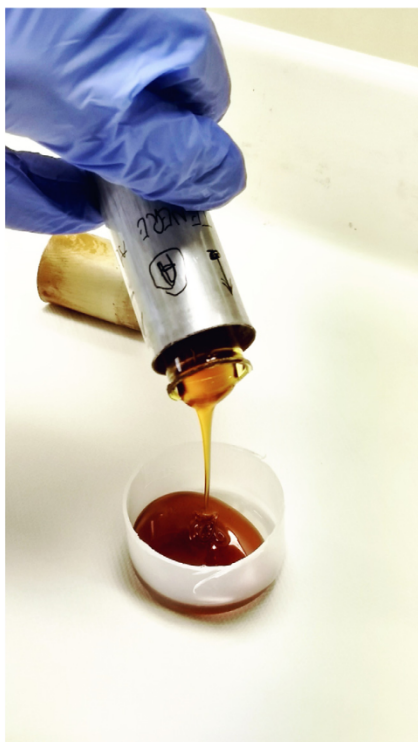
Fig. 3. Oil sample irradiated at 7.80 MGy poured from its irradiation set-up.
