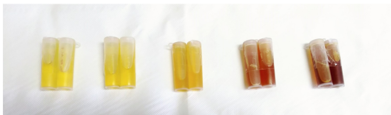
Fig. 1. Oil samples at different irradiation levels, from unirradiated (left) to 7.80 MGy (right).
